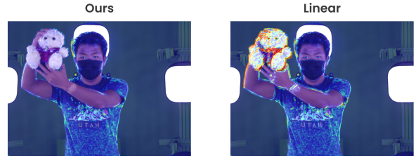
Figure 7. Ablation on spline trajectory. Without spline trajectories, the error heatmap highlights larger errors along the bear’s edges due to imprecise piecewise linear motion.
